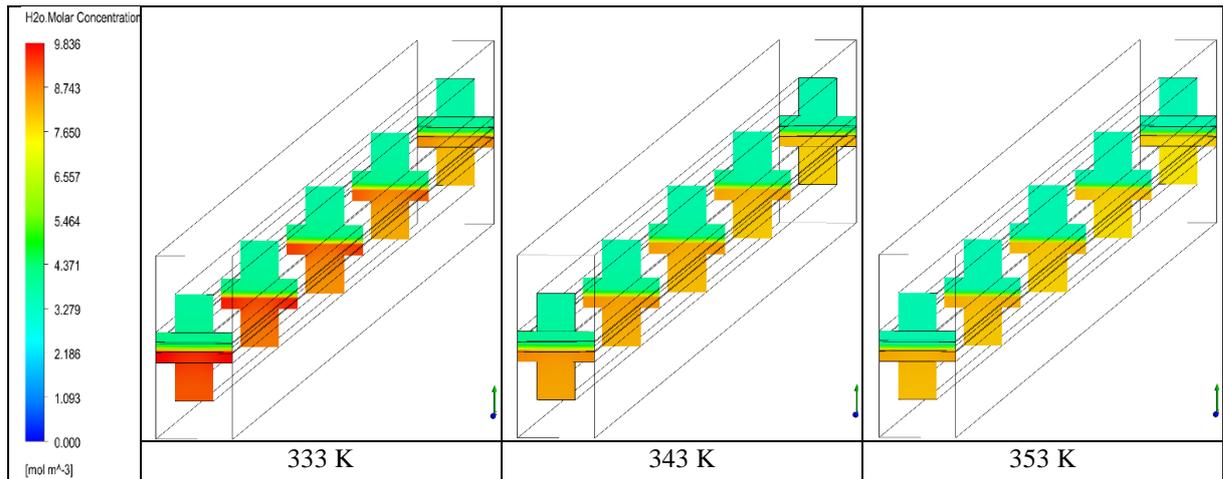
Figure 4. Water mass fraction distributions in the PEMFC single straight channels
