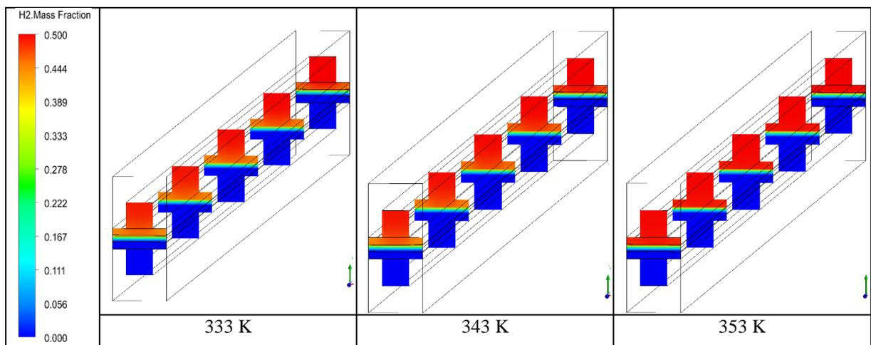
Figure 2. Hydrogen mass fraction distributions in the PEMFC single straight channels
