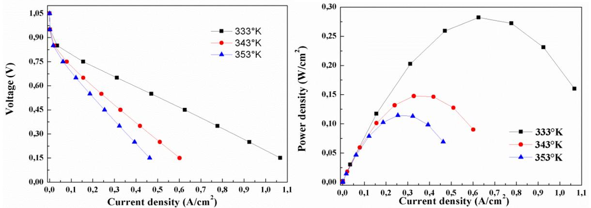
Figure 6. PEMFC polarization curves. a) Current density vs. voltage, b) Current density vs. power density
