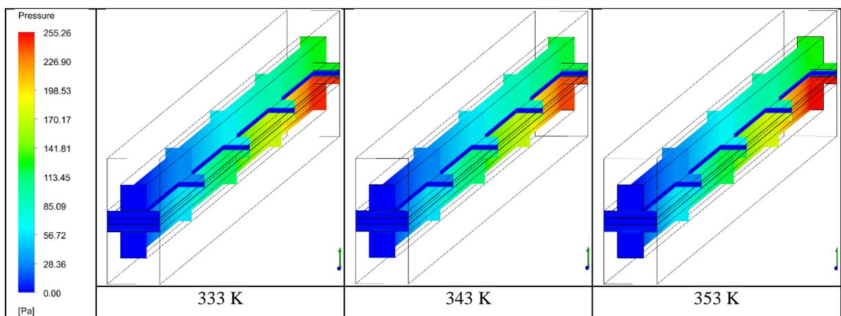
Figure 5. Pressure distributions in the PEMFC single straight channels
