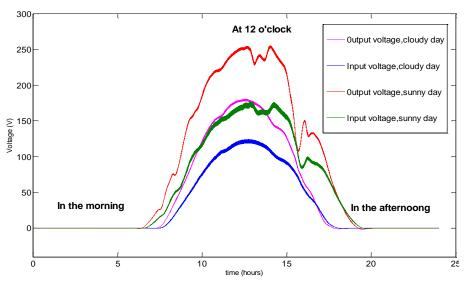
Figure 19. Evolution of input and output voltage (cloudy and sunny day)
