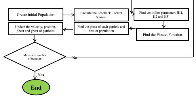
Figure 5. Flow chart of the Proposed PSO Algorithm
