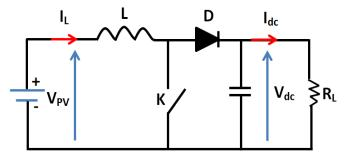
Figure 4. DC-DC Boost converter
