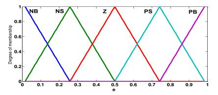
Figure 7. The Membership function of input e(k)
