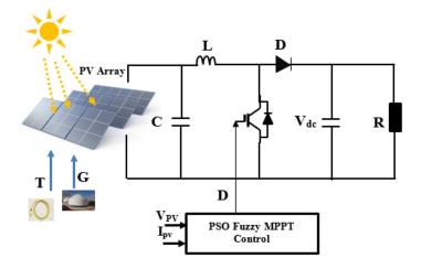
Figure 1. Stand-alone photovoltaic system.
