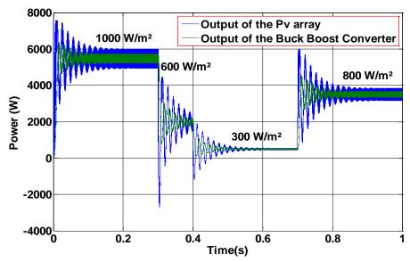
Figure 16. Output power of the PV array and boost converter at constant temperature (T=25 C°)
