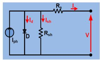
Figure 2. Typical circuit of PV solar cell.
