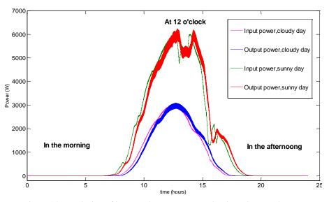
Figure 18. Evolution of input and output power (cloudy and sunny day)
