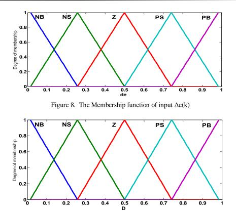
Figure 9. Membership functions of output D (Duty cycle)
