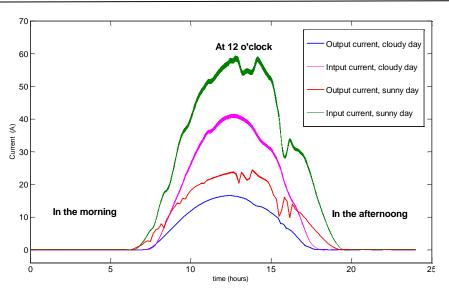
Figure 20. Evolution of input and output current (cloudy and sunny day)
