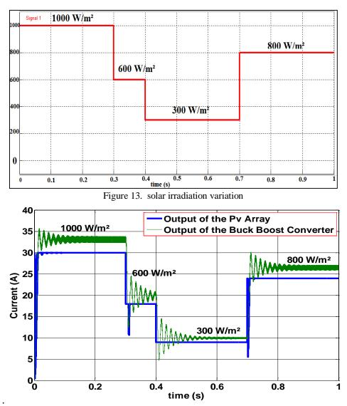
Figure 14. An output current of the PV array and boost converter at constant temperature (T=25 C°)
