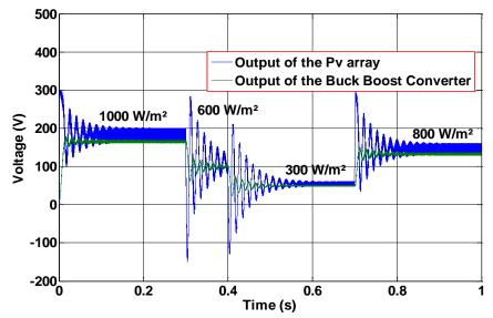
Figure 15. An output voltage of the PV array and boost converter at constant temperature (T=25 C°)
