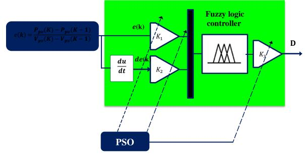
Figure 11. PSO fuzzy MPPT controller Proposed
