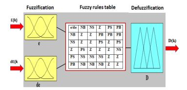
Figure 6. Fuzzy controller configuration
