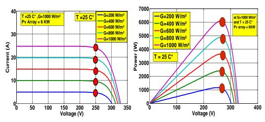
Figure 3. V-I and V-P specific of PV Array (6 kWp) under the change in irradiation
