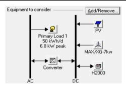
Figure 8. Configuration of the PV-wind system to be optimized.
