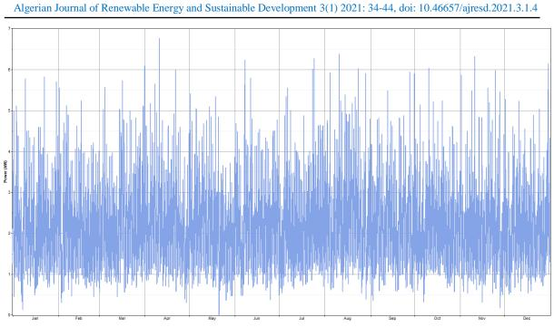
Figure 1. Load profile of the village (kW).
