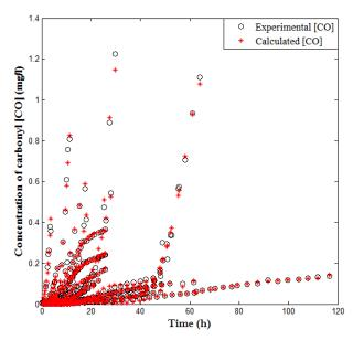
Figure 3. The comparison of experimental and calculated concentration of carbonyl [CO] as function of time.
