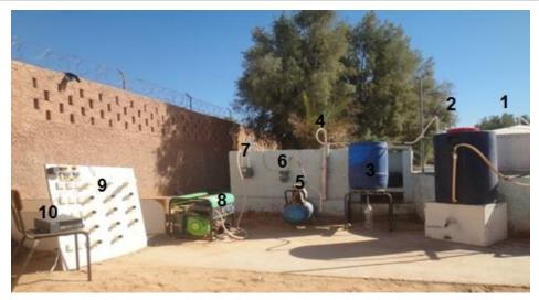
(1) Digester; (2) CO2 filter; (3) Water trap; (4) H2S filter; (5) Air compressor;
