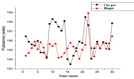
Figure 10. Power of the electric current with town gas and our biogas.
