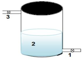
(1) Arrival of biogas; (2) lime water; (3) Exit biogas Figure 2. Descriptive diagram CO<sub>2</sub> carbon dioxide filter.
