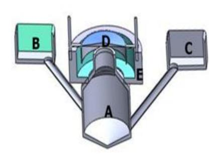
A: Digestion tank; B: Feeder tray; C: Digesta evacuation tank; D: Gasometric bell; E: Gasometer basin Figure 1. The different components of the underground digester.
