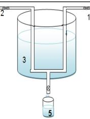
(1) Arrival of hydrated biogas; (2) Take out dehydrated biogas; (3) Ice water; (4) U shape copper tube; (5) Water recovery.
