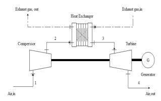
Figure 3. Basic configuration of Air Bottoming Cycle
