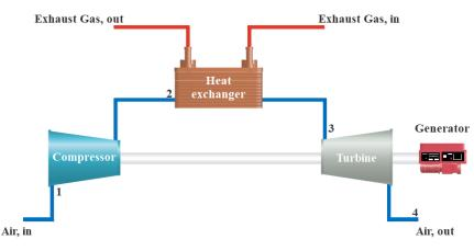
Figure 2. Air bottoming cycle scheme
