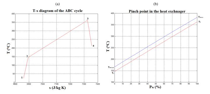
Figure 4. (a). T-S diagram of the ABC, (b). The pinch point in the heat exchanger
