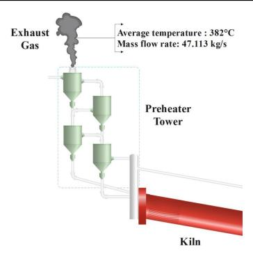
Figure1. Exhaust gas at the level of the preheater tower
