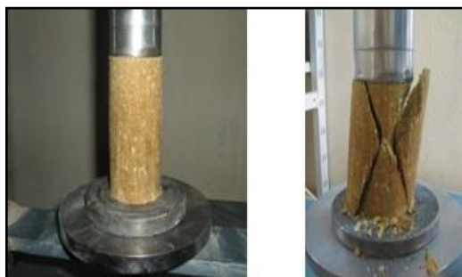
Figure 10. Test piece of tuff / sand dune mixture subjected to the compression test.
