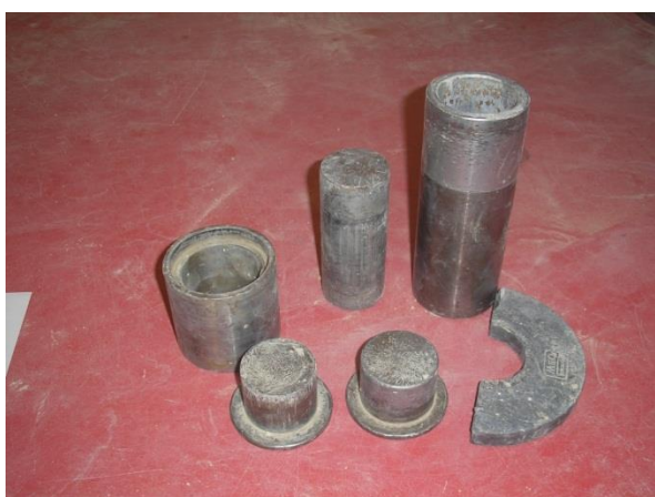
Figure 8. Test specimen mold for simple compression testing
