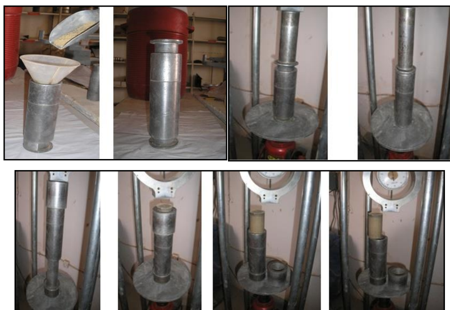
Figure 9. Steps for making cylindrical specimens for simple compression testing
