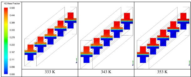
Figure 2. Hydrogen mass fraction distributions in the PEMFC single straight channels
