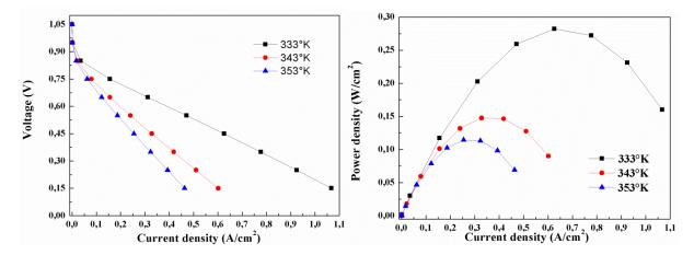
Figure 6. PEMFC polarization curves. a) Current density vs. voltage, b) Current density vs. power density
