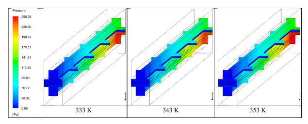
Figure 5. Pressure distributions in the PEMFC single straight channels
