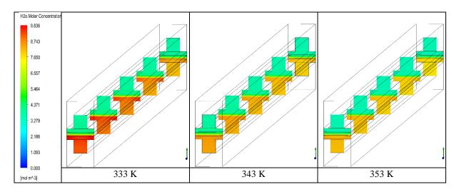
Figure 4. Water mass fraction distributions in the PEMFC single straight channels
