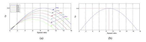
Figure 3. Power Coefficient versus tip-speed ratio for various values of  $\beta$ .
