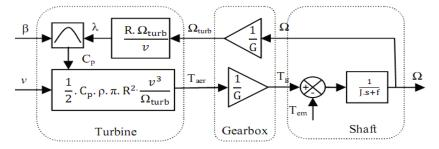
Figure 4. Wind turbine model.
