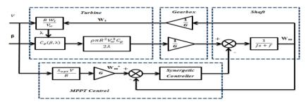
Figure. 5. MPPT-synergetic method bloc diagram.
