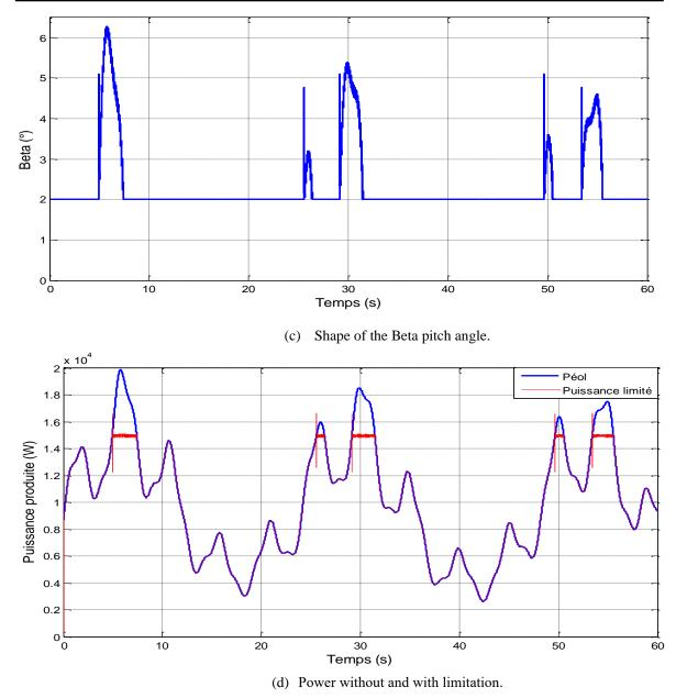
Figure 8. Results of the operatin zones with MPPT and Pitch controller.
