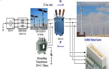
Figure 4. Model of wind energy controlled with STATCOM.
