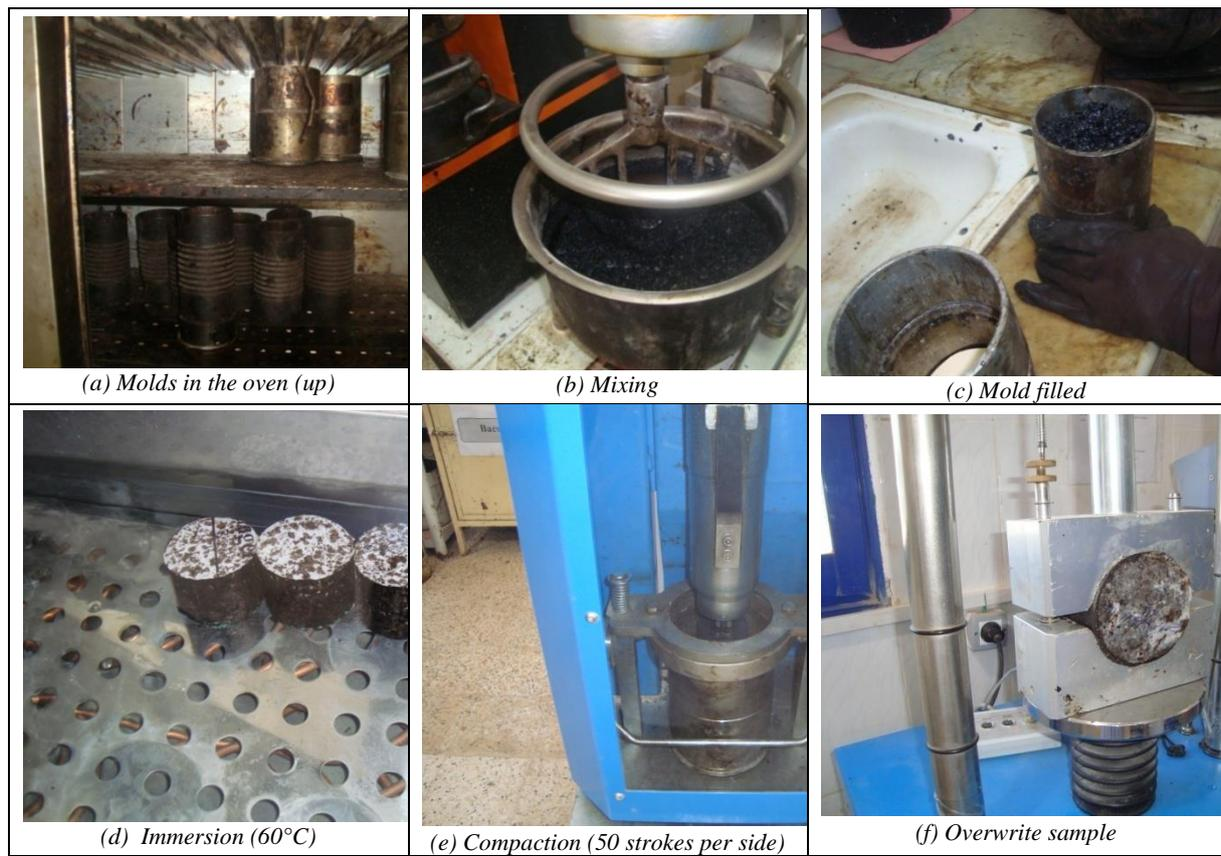
Figure 4. Stages of manufacture and storage of specimens intended for the Marshall test
