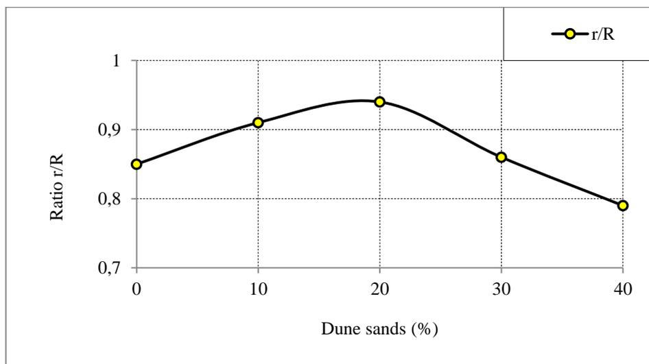
Figure 6. Effect of adding dune sands on the water resistance of asphalt mix
