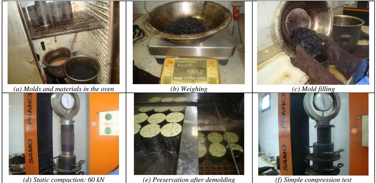
Figure 3. Stages of manufacture and storage of specimens intended for the Duriez test
