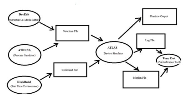
Figure 3: ATLAS inputs and outputs [11]
