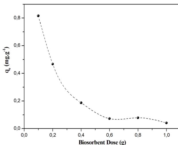
Figure 2. Effect of biosorbent dose on the adsorption capacity of MB.
