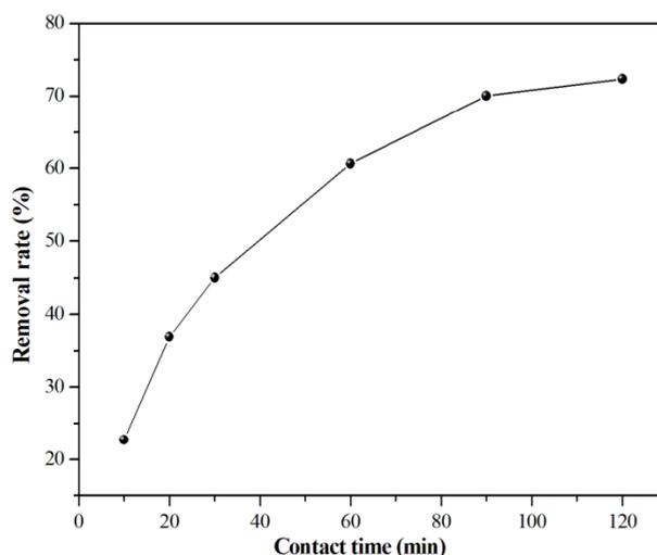
Figure 3. Effect of contact time on the adsorption of MB by prepared biosorbent.
