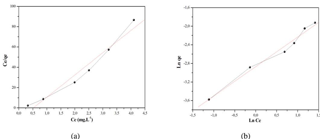
Figure 4. Langmuir isotherm of MB on the prepared biosorbent (a), Freundlich isotherm of MB on the prepared biosorbent (b)
