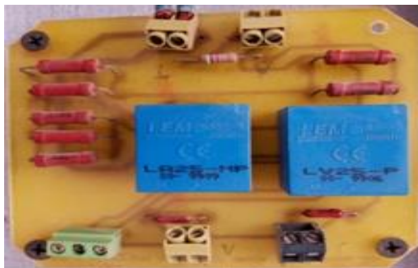
Figure 8. Sensors for measuring PV field DC current and voltage.
